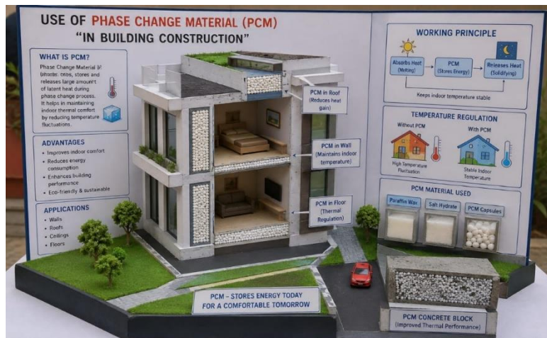
Fig 1.1- Phase Change Material in Building Construction
