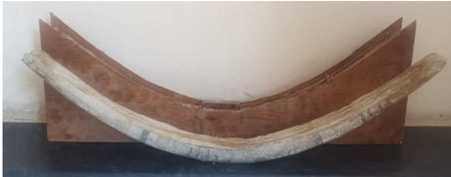
Fig.1 Mold & Leaf Spring ( Front View )
