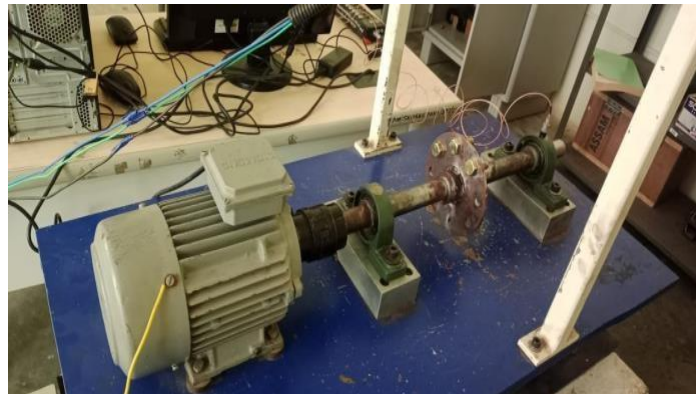
Fig. 1. Experimental Setup of Rotating Shaft with Vibration Sensors
