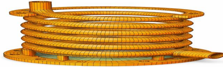
Figure 3: Computational Mesh Used for CFD Analysis
