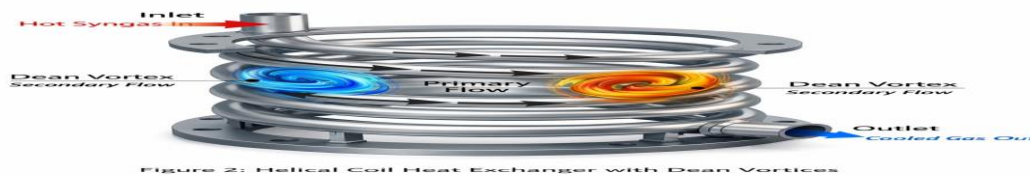
Figure 2 Helical Coil Heat Exchanger with Dean Vortices
